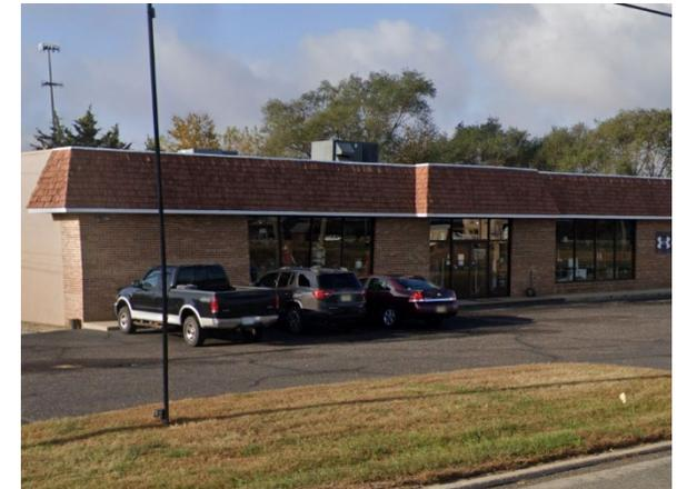
Parking spaces in the parking lot to the north of the building can be converted to porous pavement to capture and infiltrate stormwater runoff from the parking lot and rooftop. A preliminary soil assessment suggests that more soil testing would be required before determining the soil's suitability for green infrastructure.
