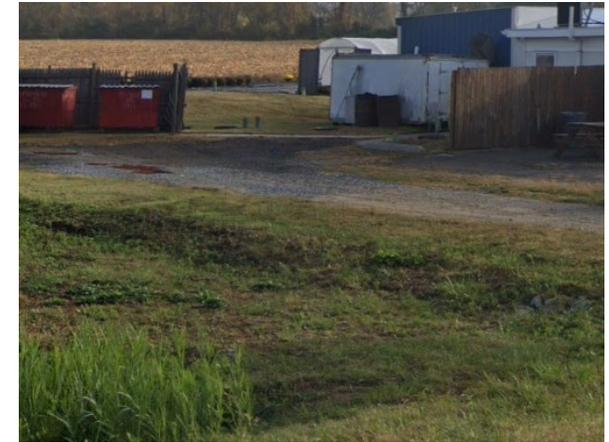
A rain garden can be installed west of the parking lot to capture, treat, and infiltrate stormwater runoff from the pavement. A preliminary soil assessment suggests that more soil testing would be required before determining the soil's suitability for green infrastructure.
